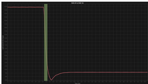
Figure 9: Asus XG27ACS, RGB 255 to RGB 102 transition with fall time marked, OSRTT Pro.
