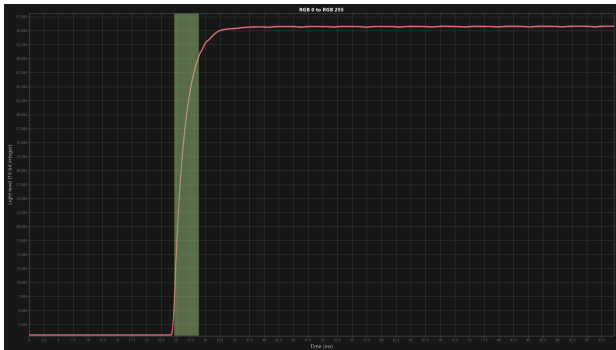
Figure 5: Asus XG27ACS, RGB 0 to RGB 255 transition with block displaying response time, OSRTT Pro.
